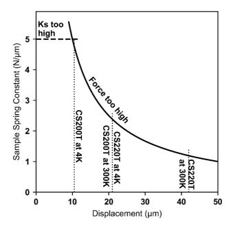
Figure 1. Recommended operating envelope for CS2x0 series cells. Sample spring constant (Ks) should be limited to about 5 N/ $\mu$ m, and force to about 50 N to avoid unwanted twisting of the cell. In other words, the sample spring constant and displacement should be chosen to lie below the solid line. Maximum displacements of the cells are marked for convenience. There is no problem using either cell at e.g. 9  $\mu$ m and 4.5 N/ $\mu$ m.
